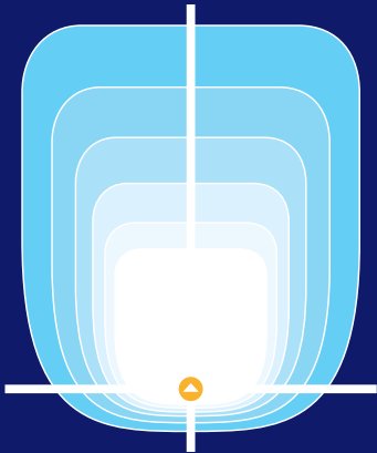
Type 4: Known as a "forward throw", or asymmetric, is best along perimeters where spill light is a concern and/or there are no places to add poles within the site.
